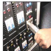
Insert at output connector to test DMX512.
