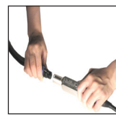
Connect both XLRs to test cable.
