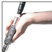
Connect one XLR to test signal.
