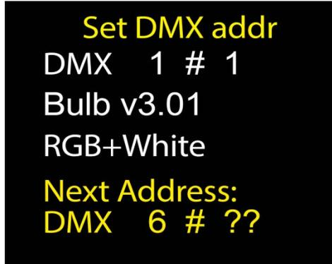
These question marks mean that the selected DMX address is not assigned to a number in a lamp chain.
