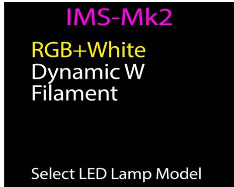
The user can change the lamp and type using the **<UP>** and **<DOWN>** buttons. When the required lamp has been chosen, press the **<SELECT>** button to activate the setting. To return to previous submenu, press the **<ESCAPE>** button.
