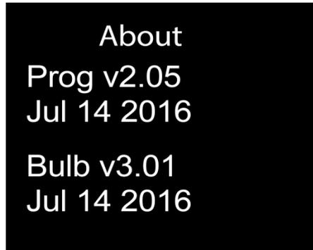
This submenu shows the current HHP software (v2.05 in this case) and the version of the firmware that will be programmed into lamps (v3.01 in this case).
