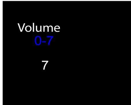
This setting sets the HHP sound volume (the HHP makes a sound notification when the device is turned on or when a lamp has been programmed).
